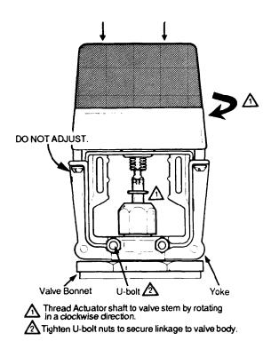
FIG. 4 -- ASSEMBLY OF ML7984 TO VALVE.
